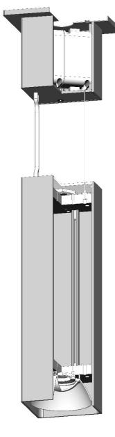
canopy mounted drivers, constant current, field maintainable, universal input (120-277v), 0-10v controllable to 5% dimming
